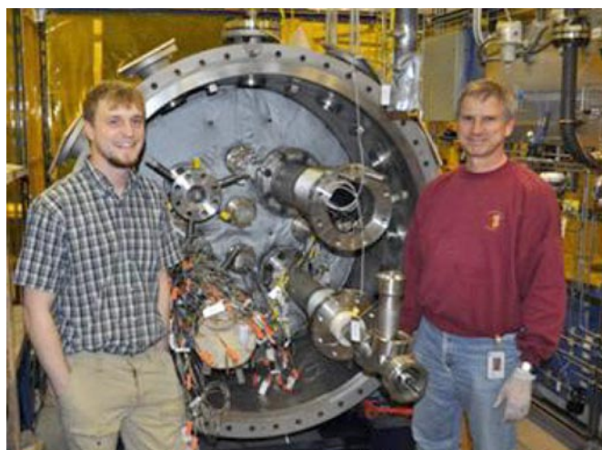
FIGURE 1. SBTS Vessel Assembly Prior to Install of the Outer Vessel Head
