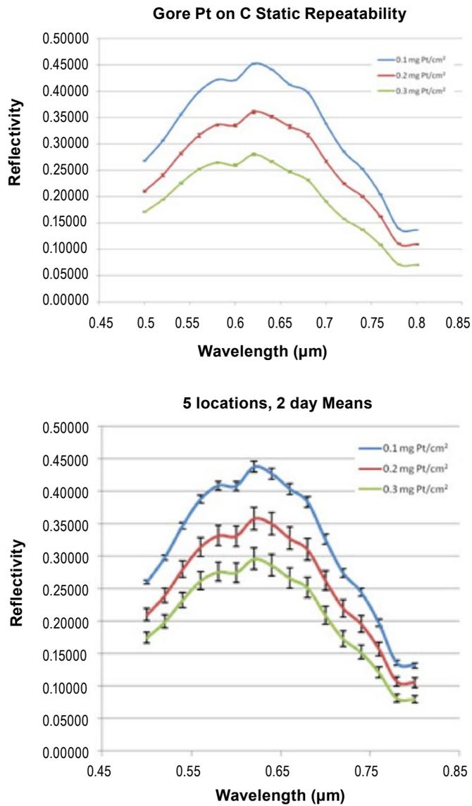
**FIGURE 3.** The plot on the top shows static repeatability data, looking at one location on each loading sample numerous times. The plot on the bottom is localized variation data, looking at five different locations on each loading sample over multiple days.
