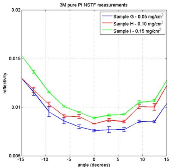
**FIGURE 1.** 3M NSTF pure Pt sample loading data. The separation between the curves relative to the error bars is a measure of the sensitivity.
