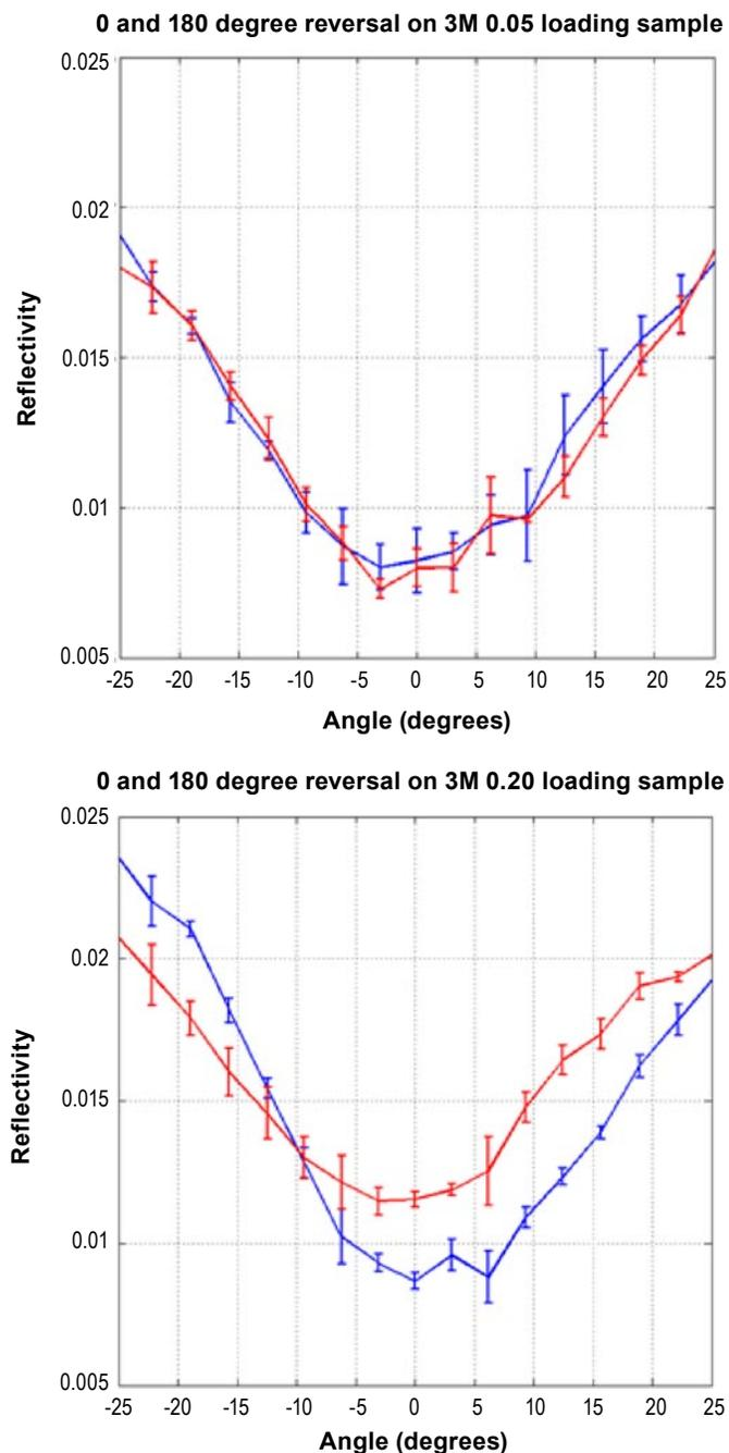
**FIGURE 2.** The plot on the top is the 0 and 180 degree reversal data for the  $0.05 \text{ mg/cm}^2$  sample. The plot on the bottom is the 0 and 180 degree reversal data for the  $0.20 \text{ mg/cm}^2$  sample, which displays the asymmetric behavior.
