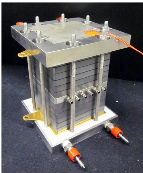
FIGURE 1. Fuel cell stack for testing 50 cm 2 MEAs produced using thermal pressing, thermal pressing with APC, and ultrasonics.
