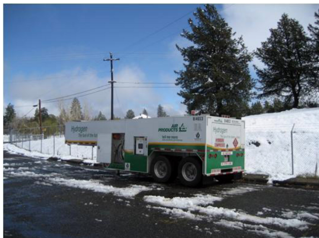
FIGURE 6. HF-150 Mobile Refueler at the District Office of the U.S. Forest Service in Placerville, California
