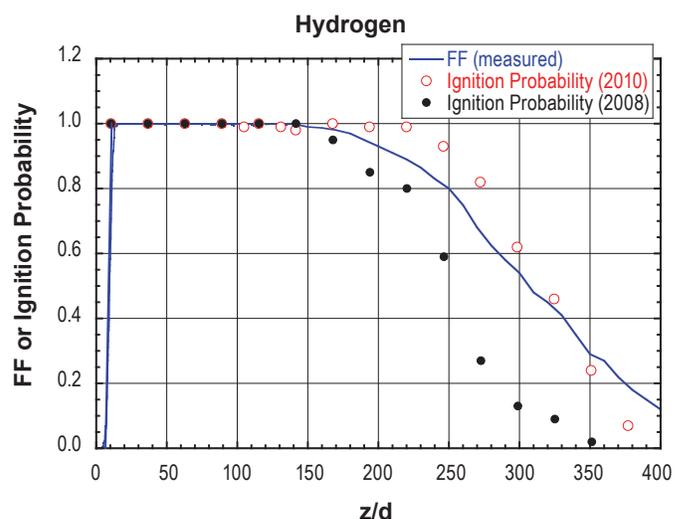
FIGURE 1. Original and Repeated Centerline Profile FF and Laser Spark Ignition Probability Measurements
