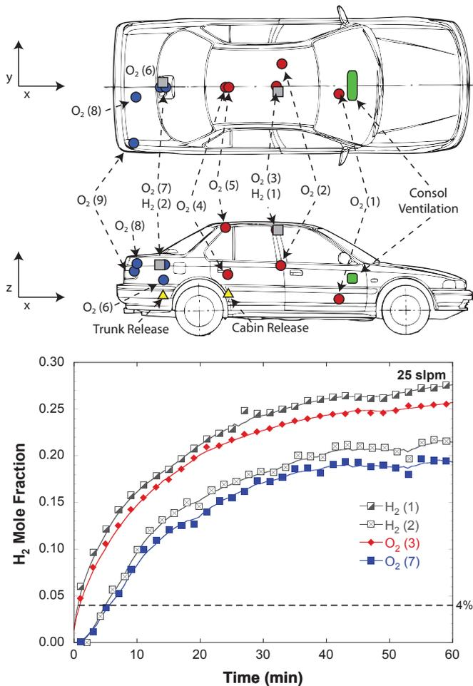
**FIGURE 3.** Schematic of trunk O<sub>2</sub> (blue), passenger cabin O<sub>2</sub> (red), and H<sub>2</sub> sensors (grey), along with ventilation (green) and release (yellow) points within the simulated fuel cell vehicle. Data shows a comparison of volumetric concentration measurements from co-located H<sub>2</sub> and O<sub>2</sub> sensors in the trunk and passenger cabin for the baseline condition.
