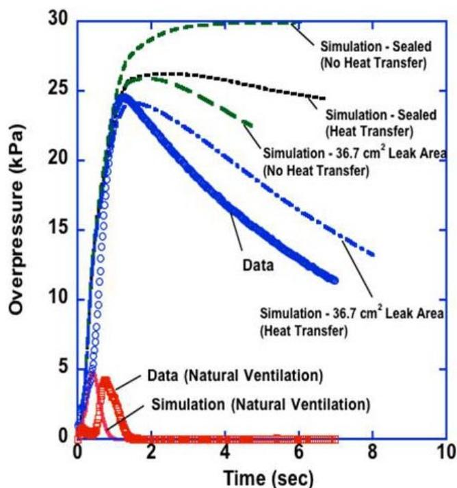
**FIGURE 4.** Comparison of Measured Ignition Overpressure in the SRI International Subscale Warehouse Facility with Results from FUEGO/FLACS Model Simulations
