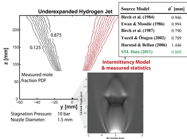
**FIGURE 2.** Flammability factor maps for the choked hydrogen jet ( $p_0/p = 10$ ,  $d = 1.5$  mm), with black contours generated from direct PDF integration, while red contours were generated from concentration statistics and an applied intermittency model. A schlieren image of jet exit shock structure is shown at the bottom, while tabulated predictions (black) and measurements (green) of the effective source diameter are shown to the right.
