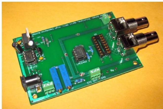
**FIGURE 4.** Custom-designed sensor impedance buffer circuit to isolate electrochemical sensor from external electrical influences. Photograph provided by Custom Sensor Solutions, Inc.
