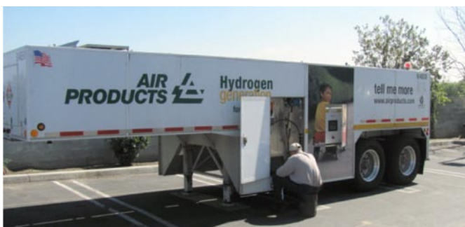
FIGURE 2. Air Products Mobile Refueler Servicing the Two H 2 Buses
