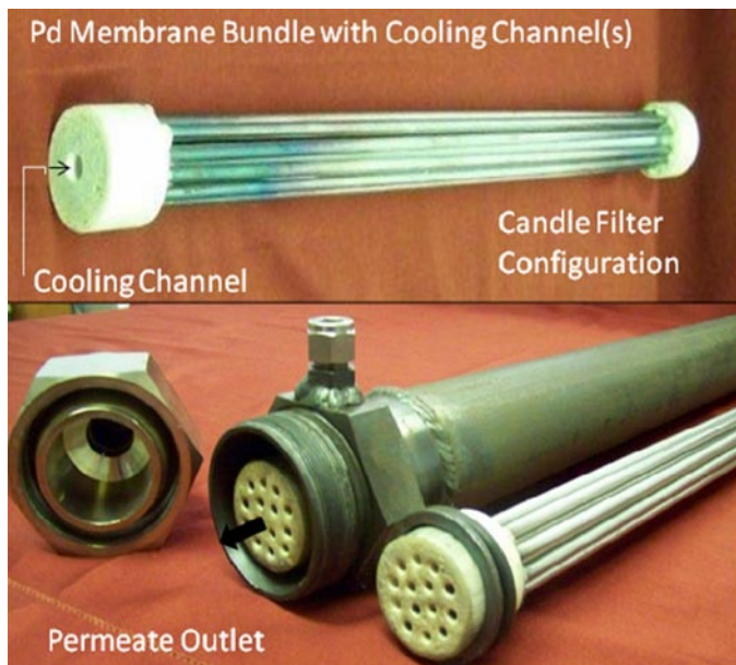
FIGURE 3. Fabrication of a Membrane Reactor for Pd Ceramic Composite Membrane with Integral Cooling Coil for the Target Exothermic WGS Reaction
