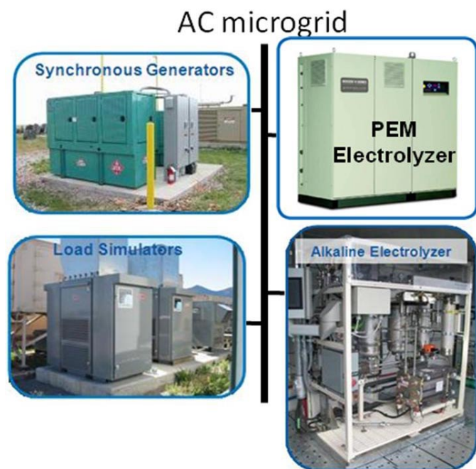
FIGURE 1. Frequency regulation experimental system where electrolyzers are powered by diesel generators on an AC microgrid
