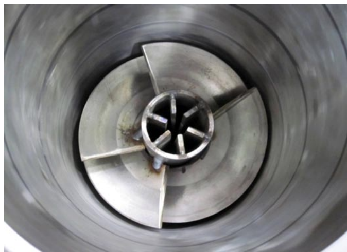
FIGURE 2. Nested auger design prototype for particle conveyance
