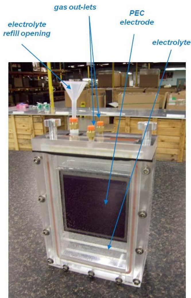
FIGURE 3. Prototype PEC module design with four inch by four inch PEC electrodes
