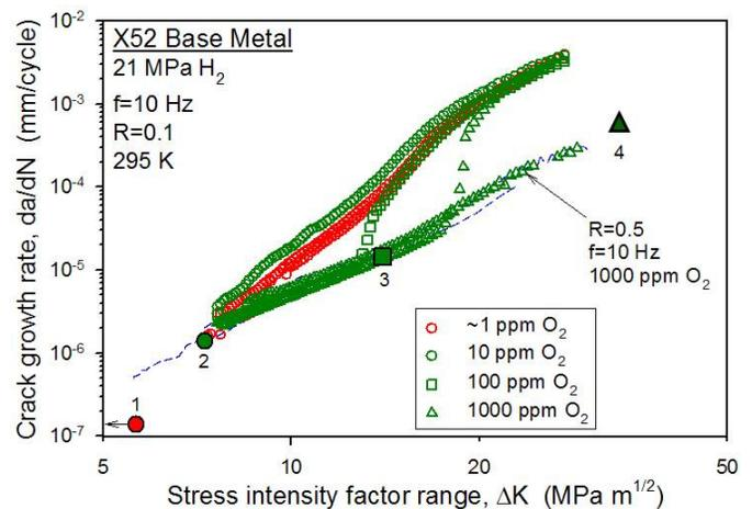
**FIGURE 1.** Fatigue crack growth rate (da/dN) vs stress-intensity factor range ( $\Delta K$ ) data for X52 steel in  $H_2/O_2$  gas mixtures, high-purity hydrogen, and air. The symbols labeled 1, 2, 3, and 4 represent model predictions for the mechanical da/dN level required for  $\theta_0 < 1$ .
