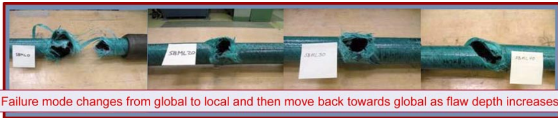
FIGURE 2. Photo Illustrating Failure Mode of FRP
