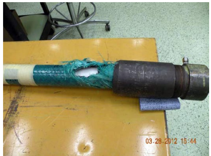
FIGURE 4. Burst Failure Following 8077 Rated Pressure Fatigue Cycles
