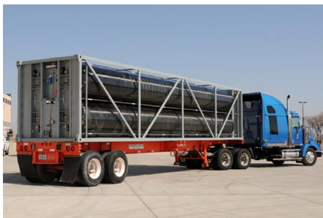
FIGURE 1. Assembled ISO Container without Outer Panels
