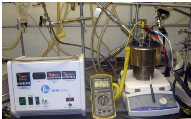
FIGURE 1. The modified Parr reactor as a pressurized electrochemical cell shown as it looks in operation. With factory-sealed electrodes and Swagelok fittings, this reactor is rated to 2,500 psig operating pressure.
