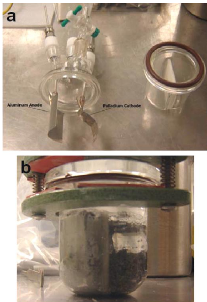
FIGURE 4. a) Showing a glass frit-divided electrochemical cell with an aluminum anode and palladium cathode in place. b) The saturated LAH-THF solution forces the alane-THF adduct to precipitate at the anode as a grey-white solid.
