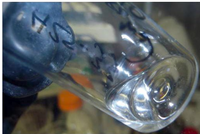
FIGURE 2. 1:1 molar mixture of hexyl-AB, heated for 12 h @ 130^\circ\text{C} . Picture was acquired at room temperature.
