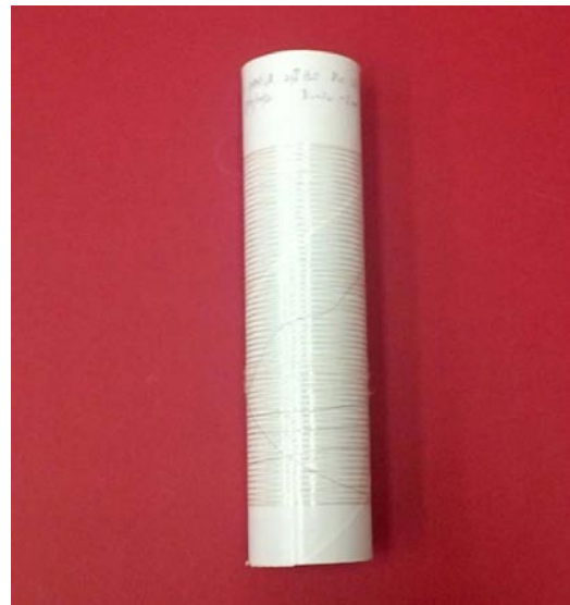
FIGURE 2. Melt-spun PAN/VT fibers generated with new system/winder with traverse fiber guide
