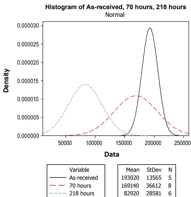
**FIGURE 3.** Probability distribution of cycles to failure (as-received MEA; cell run for 70 hours in membrane combined chemical-mechanical AST, and cell run for 218 hours in membrane combined chemical-mechanical AST)
