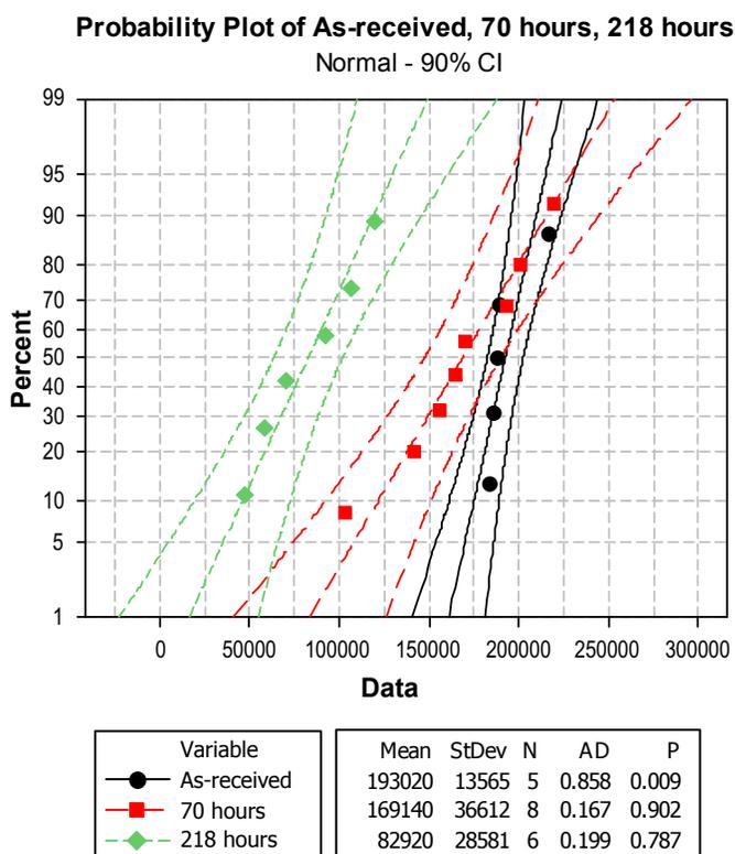
**FIGURE 4.** Comparison of cumulative probability distribution of the cycles to failure (as-received MEA; cell run for 70 hours in membrane combined chemical-mechanical AST, and cell run for 218 hours in membrane combined chemical-mechanical AST)
