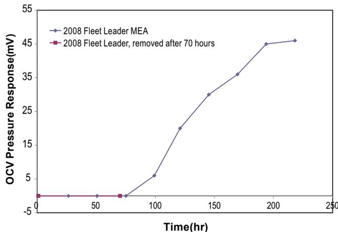
FIGURE 2. OCV pressure response during membrane combined chemical-mechanical AST
