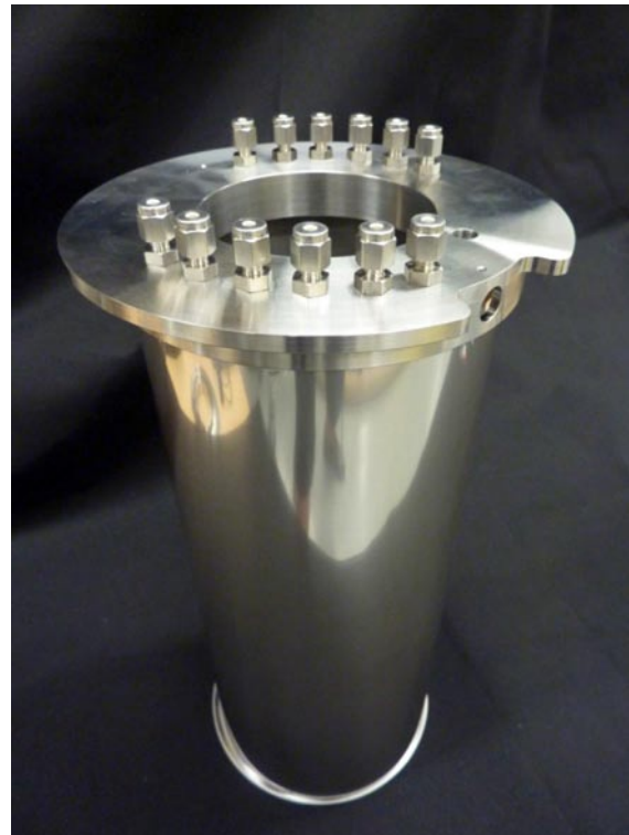
FIGURE 3. InnovaTek proprietary catalytic steam reforming reactor
