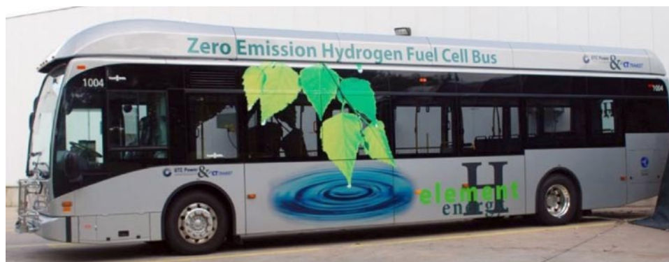
FIGURE 2. The bus pictured, which is in service at CTTRANSIT in Hartford, Connecticut, is a fuel cell dominant Van Hool 40-foot bus with a UTC Power Fuel Cell System, Seimens ELFA hybrid system using lithium-based batteries
