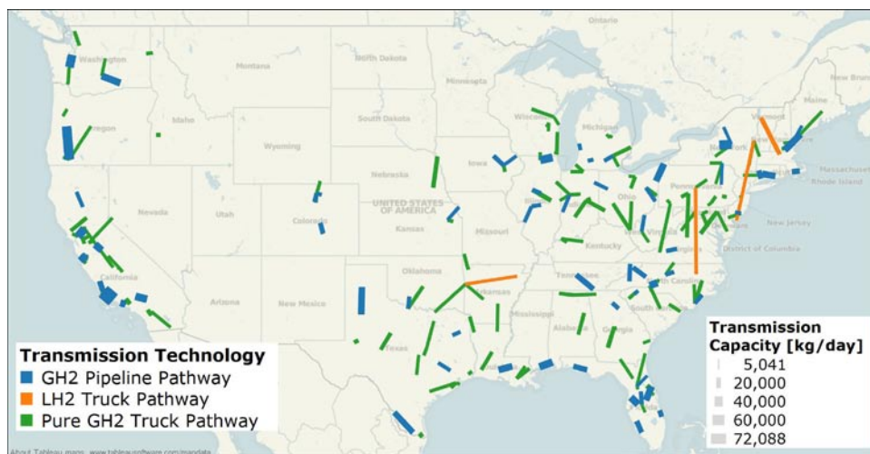
FIGURE 3. Transmission infrastructure build-out under the early-market “hydrogen success” scenario
