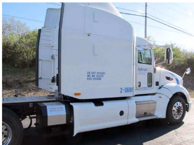
FIGURE 2. Delphi SOFC APU (B-Level Prototype) Installed on PACCAR Truck
