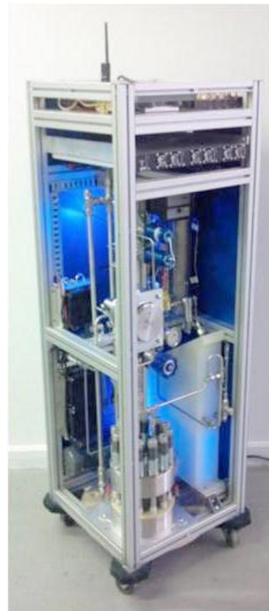
FIGURE 3. Electrolyzer (HRA) System
