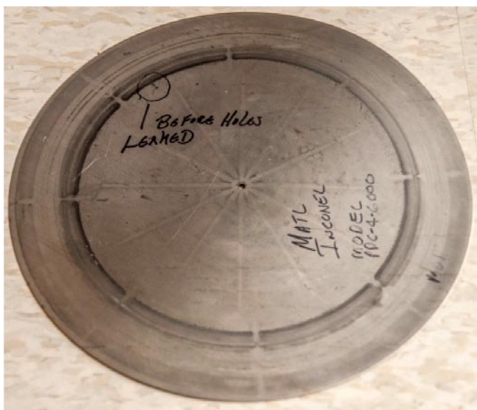
FIGURE 1. Picture of a PDC diaphragm taken out of service, showing the ring of black deposit suspected to be a cause in reduced diaphragm life. The location of the crack, where the diaphragm leaked, is circled with a black marker.
