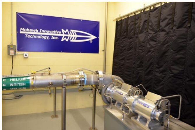
FIGURE 2. MiTi® Single-stage compressor system with high speed oil-free motor drive.
