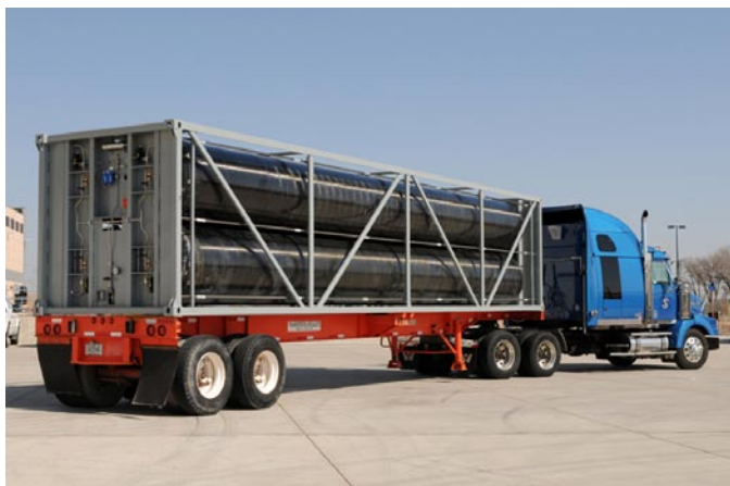
FIGURE 1. Assembled TITAN™ ISO Container (without outer panels) on Standard ISO Trailer
