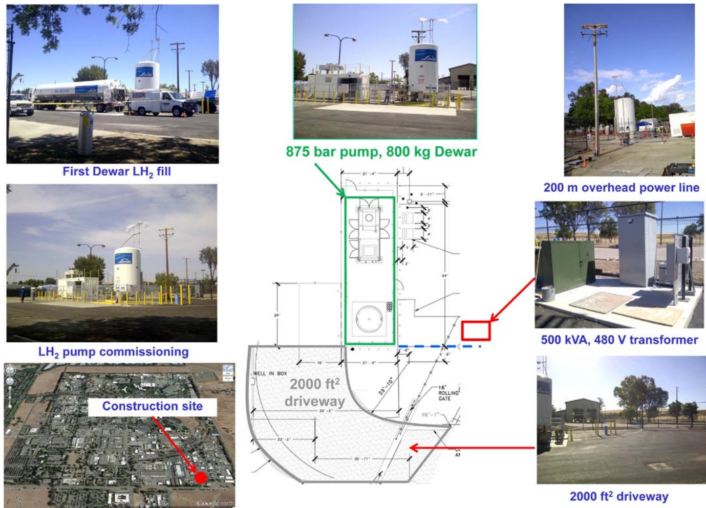
FIGURE 1. Construction-ready liquid hydrogen pump site drawing including pictures of the main features and events leading to pump commissioning.
