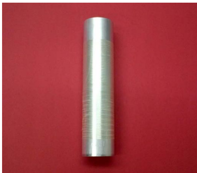
FIGURE 2. Drawn PAN/VT Fibers Generated with Water and Acetonitrile
