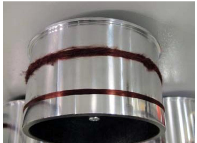
FIGURE 6. Top: “Fuzzing” of Filament Tow during Oxidative Stabilization. Bottom: Tow not exhibiting “Fuzzing”
