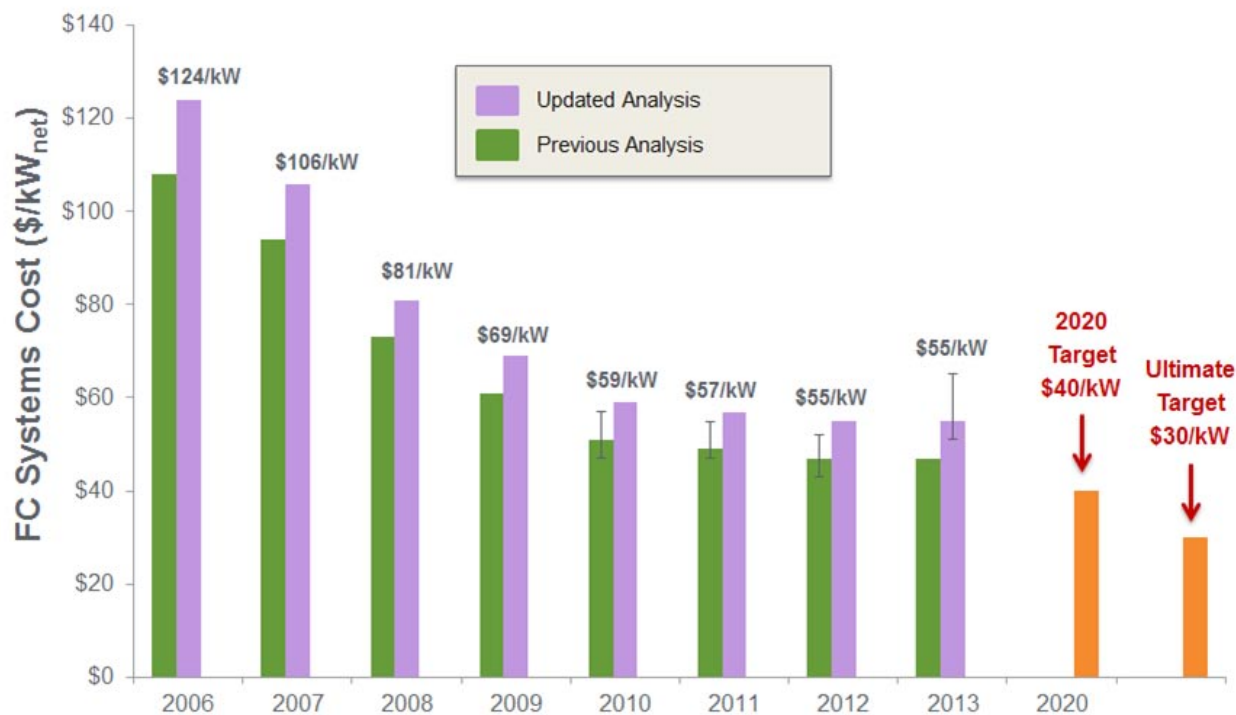
Figure 1. Modeled cost of an 80-kW automotive fuel cell system based on projection to high-volume manufacturing (500,000 units/year). 2
