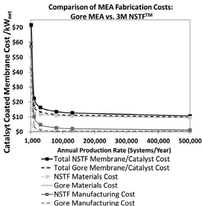
**FIGURE 1.** Cost Comparison of Gore and 3M MEAs
