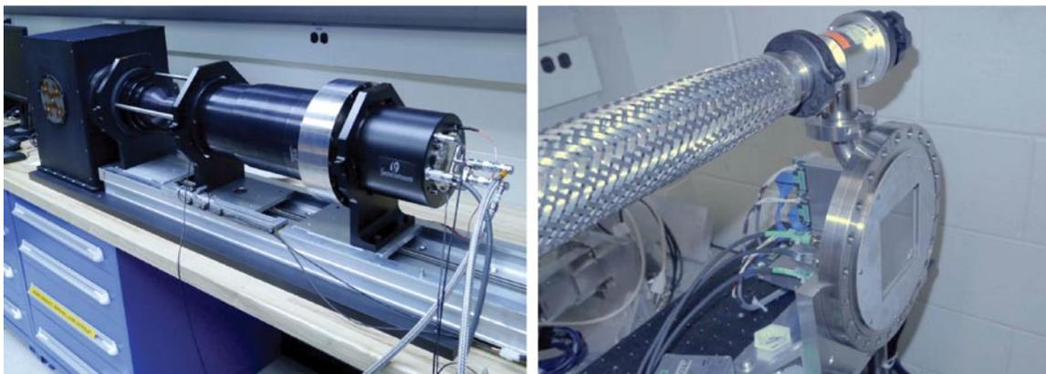
**FIGURE 1.** New large-area high-resolution detectors for validation of down the channel models of fuel cell operation.
