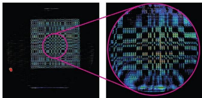
**FIGURE 2.** Contact radiograph of test pattern on left. Magnified 4x neutron image of test pattern on right.
