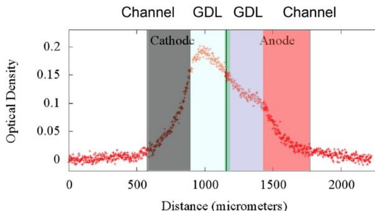
**FIGURE 3.** Left lens 4x magnified image of a dry fuel cell, right optical density is plotted, which is proportional to the water thickness. An additional calibration measurement is required to accurately convert to water thickness, but was not performed to limited beam time.
