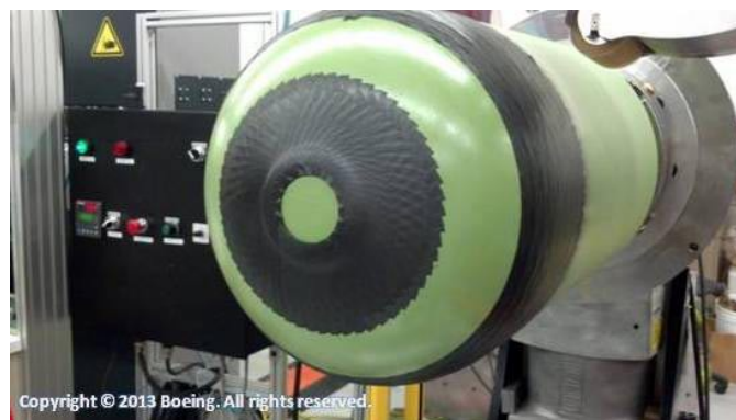
FIGURE 1. Layup of Aft Dome Cap on Foam Mandrel—the Mandrel has a Released Coating (Green) to Facilitate the Removal of the Layup
