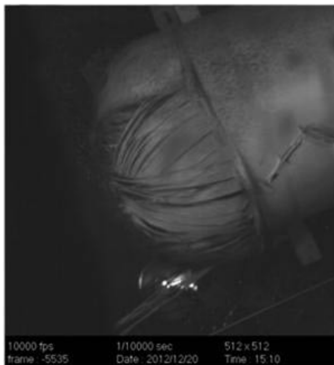
FIGURE 3. Vessel 13 Burst Test High-Speed Video Frame
