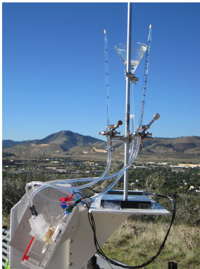
FIGURE 1. Photograph of the photoreactor mounted on a solar tracker. A cylindrical lens was affixed to the front window and focused the sunlight onto the semiconductor photoelectrode. Captured hydrogen and oxygen gas was measured in inverted pipettes to determine the Faradaic yield over the 4-hour test runs.
