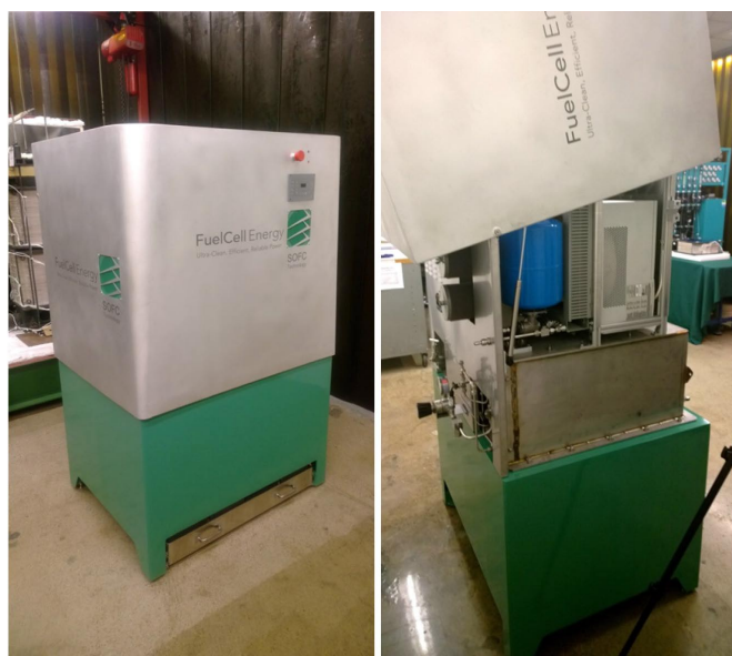
FIGURE 3. FCE's Integrated 2-kW e Bio-Fueled SOFC Skid
