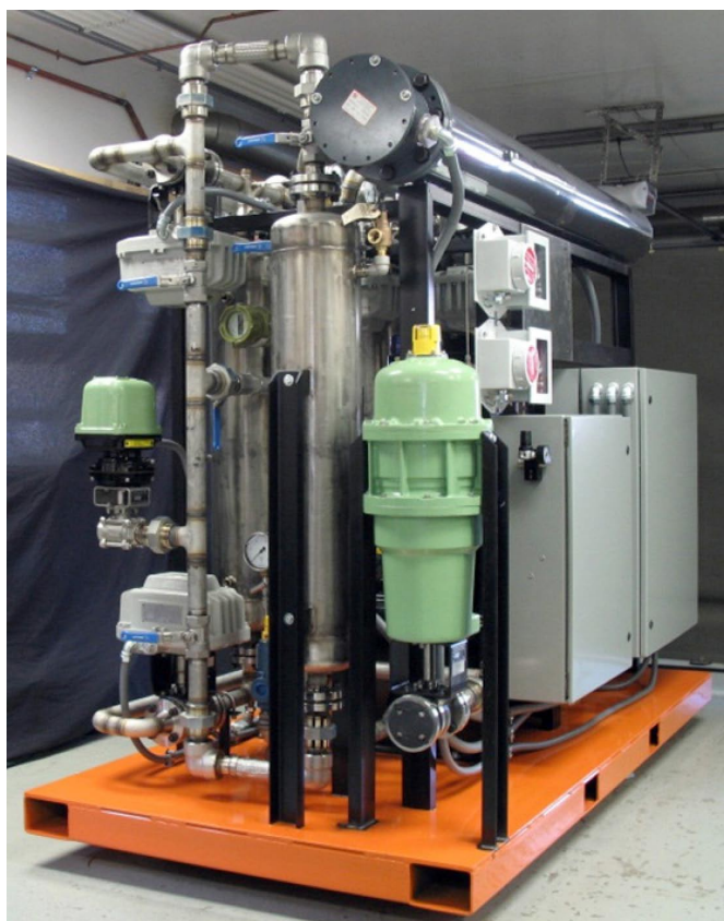
FIGURE 2. TDA's Biogas Clean-Up Skid
