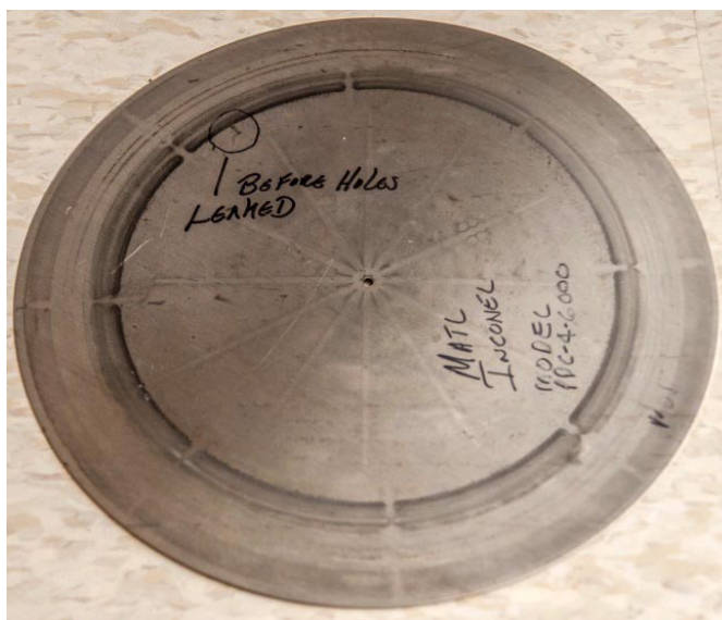
FIGURE 1. Picture of a PDC diaphragm taken out of service, showing the ring of black deposit suspected to be a cause of reduced diaphragm life. The location of the crack, where the diaphragm leaked, is circled with a black marker.
