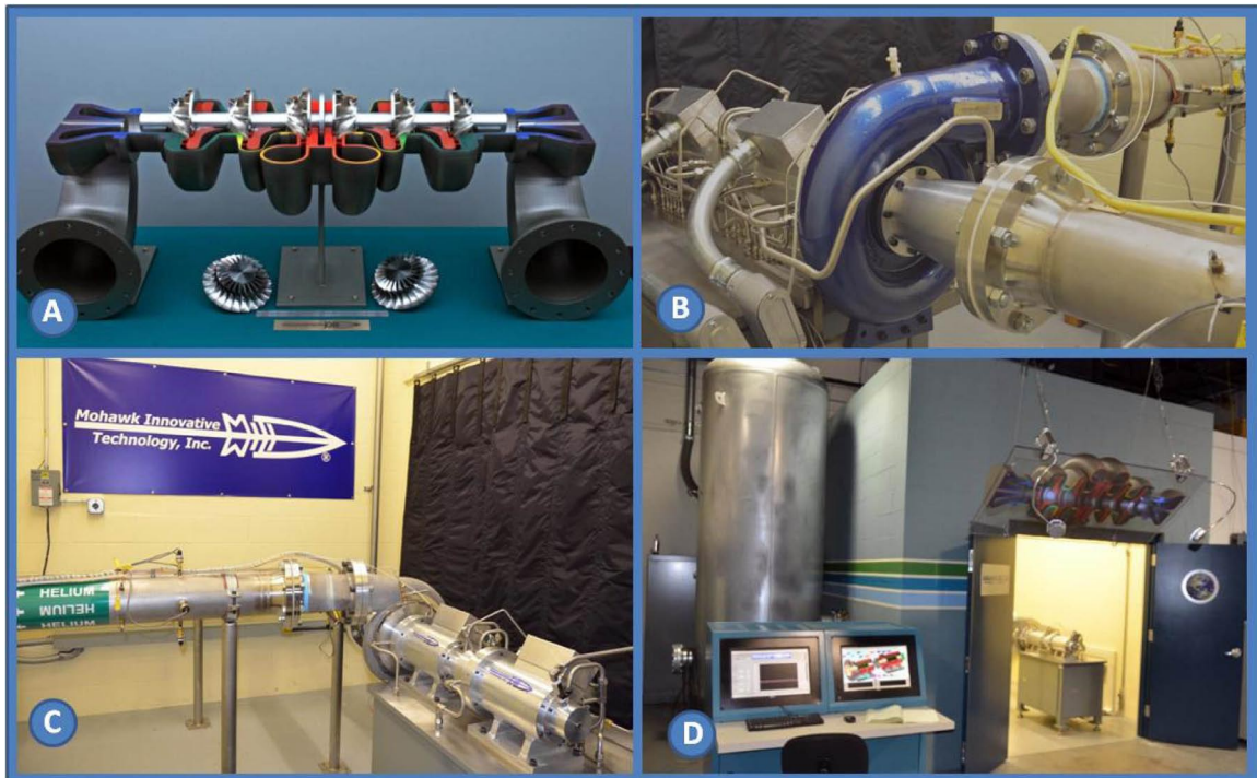
FIGURE 1. MiTi® Single-Stage Compressor System with Oil-Free, 60,000 RPM Motor Drive and Closed-Loop Helium Test Facility
