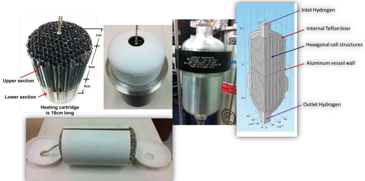
FIGURE 2. 2-Liter HexCell Prototype Assembly and Computational Model
