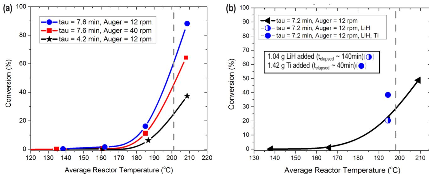
**FIGURE 2.** (a) Alane conversion as function of reactor temperature, space-time ( $\tau$ ), and auger speed for a 50 wt% alane slurry in silicon oil and (b) alane conversion as a function of reactor temperature, lithium hydride dopant, and titanium dopant for a 60 wt% alane slurry in mechanical pump fluid.
