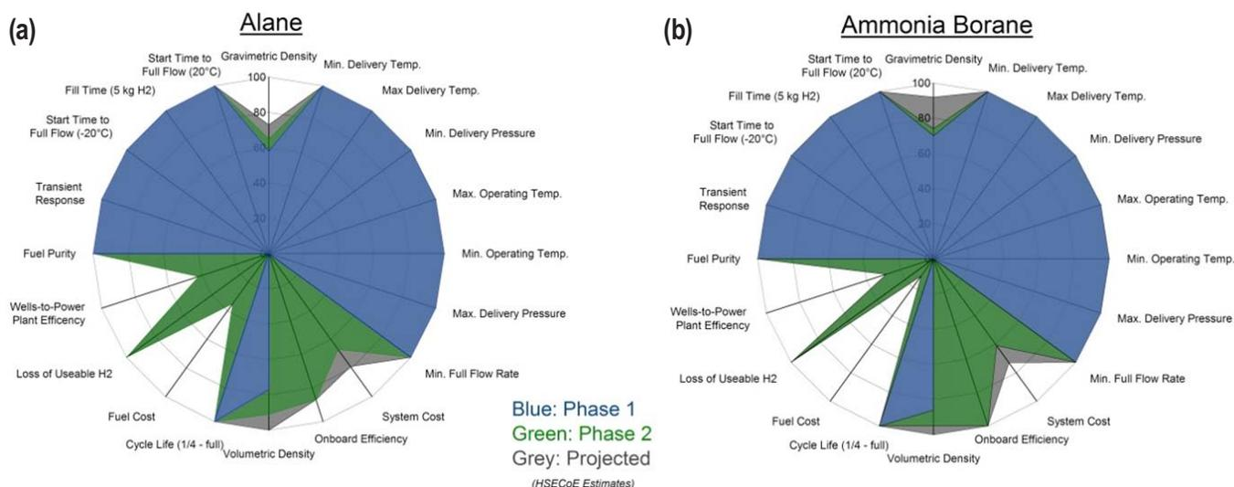
**FIGURE 1.** Spider chart summarizing our progress in meeting the DOE 2017 technical targets for (a) 50 wt% alane slurry and (b) 50 wt% ammonia borane slurry (note: values are Hydrogen Storage Engineering Center of Excellence estimates).
