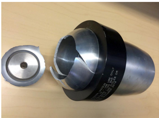
FIGURE 2. Tank after Cryo Burst
