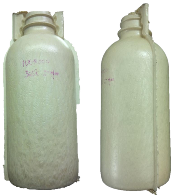
FIGURE 3. Images of a stretch blow-molded HX-8000 bottle showing the weld lines at mold interfaces. Blow-up ratio (bottle diameter to parison diameter) of 1.75.
