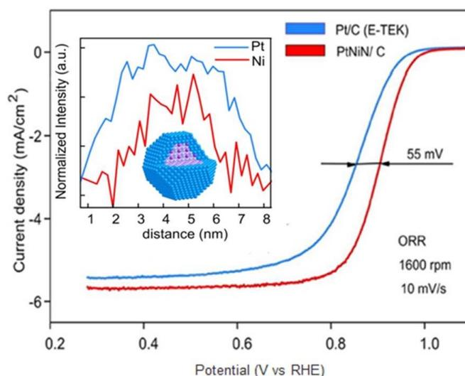
**FIGURE 3.** ORR polarization curves of PtNiN/C and Pt/C catalysts on a rotating disk electrode in 0.1 M  $\text{HClO}_4$ . Also shown is electron energy loss signal line-scan profiles of Pt and Ni in a single PtNiN nanoparticle (blue, Pt; gray, Ni; purple, N).
