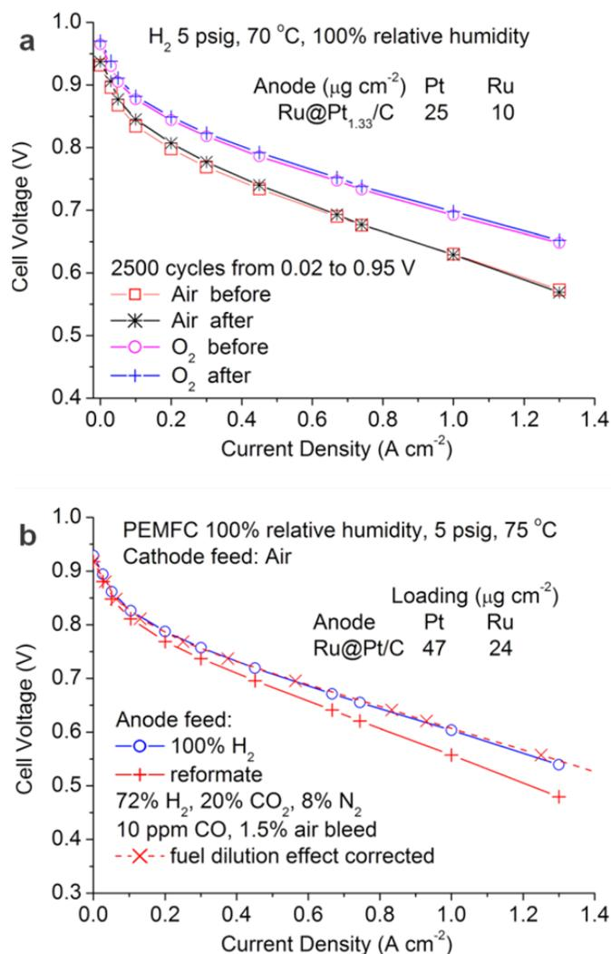
**FIGURE 2.** Results on anode durability (a), and CO tolerance (b) test for atomically perfect Ru(core)-Pt(shell) nanocatalysts.
