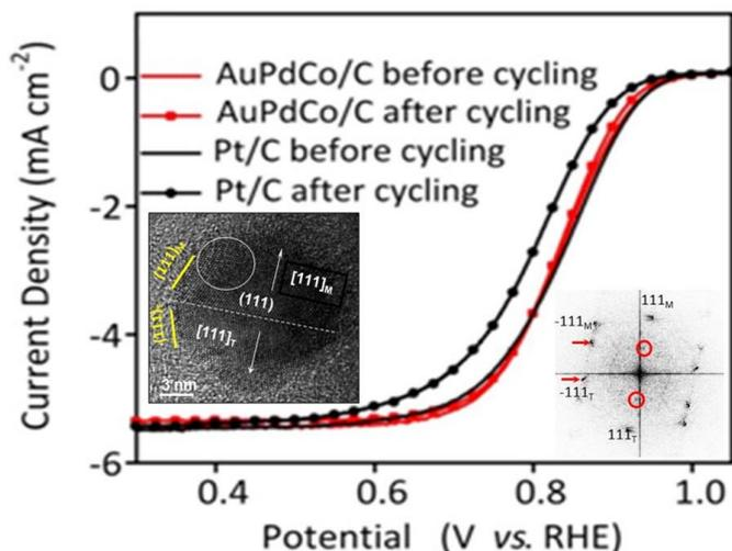
**FIGURE 4.** ORR polarization curves of AuPdCo/C-intermetallic and Pt/C catalysts before and after 10,000 cycle test between 0.6 and 1.0 V in 0.1 M KOH. Also shown is a high-resolution transmission electron microscope image and its diffractogram of a single AuPdCo intermetallic particle. Superlattice spots are visible in the diffractogram as indicated by the red circles.
