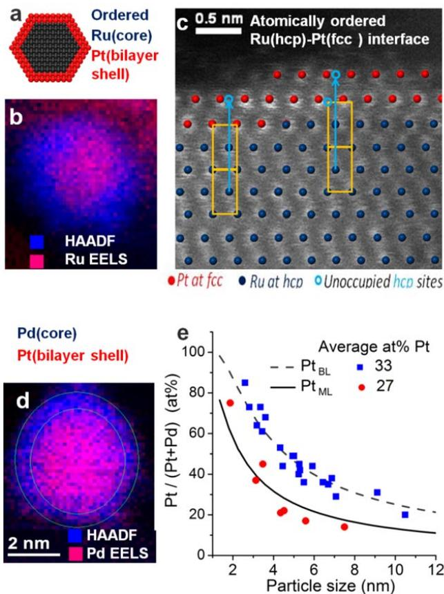
**FIGURE 1.** Structural schematics (a) and scanning transmission electron microscopy data for atomically perfect Ru(core)-Pt(bilayer shell) nanoparticles (b,c), and for Pd(core)-Pt(shell) nanoparticles (d,e).
