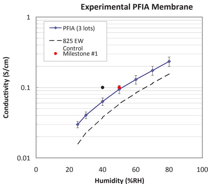
**FIGURE 2.** Conductivity versus RH for three lots of PFIA membrane with 95% confidence intervals. Standard 825 EW membrane indicated by dashed line. Project milestones indicated with circles.
