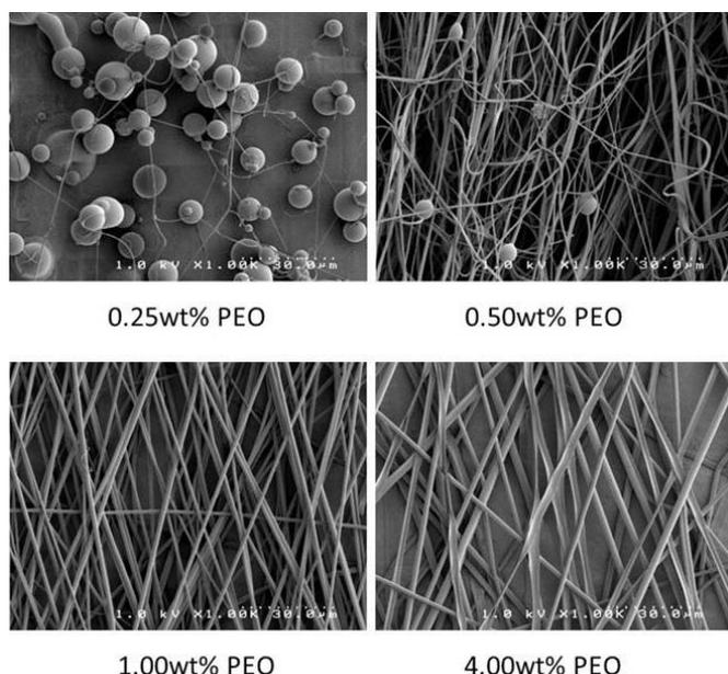
**FIGURE 4.** Electron microscope images of PFIA electrospinning experiments showing the effect of added polyethylene oxide (contribution from Vanderbilt University).
