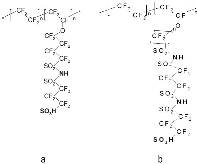
**FIGURE 1.** Multiacid side chain structures; a) PFIA and b) Perfluoroionene chain extended ionomers.
