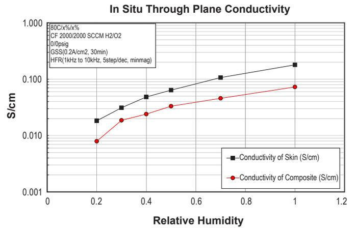
**FIGURE 3.** Through plane conductivity versus RH measured in-cell with contributions from the center composite layer decoupled from pure ionomer skin layer.
