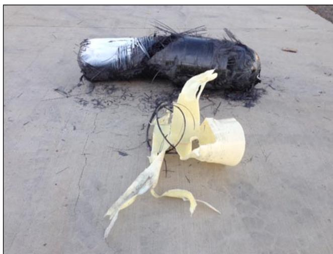
FIGURE 2. Vessel 15 Post Burst Test
