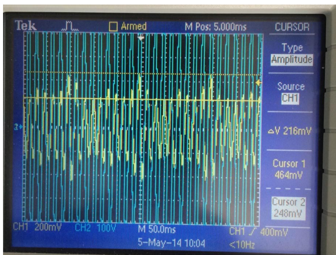
FIGURE 2. An oscilloscope was placed on the motor supply circuit to show voltage (cyan) to be uniform and current (yellow) to be variable over multiple periods.
