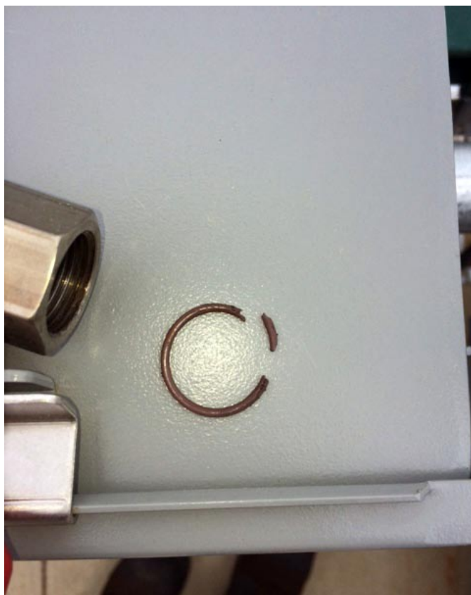
FIGURE 4. The seal on the second stage discharge check valve failed and required replacement at 60 hours.
