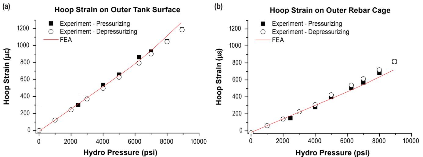
**FIGURE 4.** Comparison between experimentally measured and finite element analysis predicted strains during hydrostatic testing: (a) hoop strain on the outer surface of the steel vessel; (b) hoop strain on the outer rebar cage
