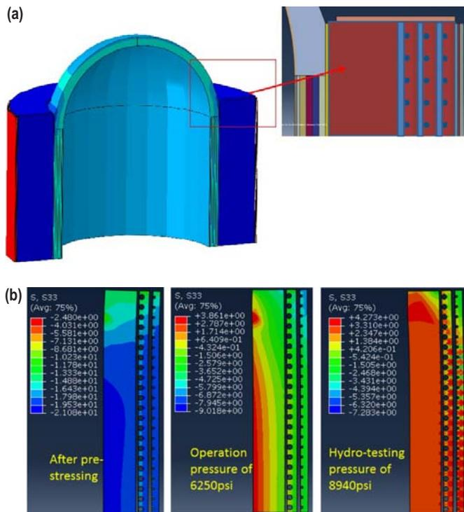
FIGURE 2. (a) Finite element model used to optimize the SCCV design; (b) Hoop stress distribution in the concrete after prestress applied, at operation pressure, and at the hydrostatic test pressure
