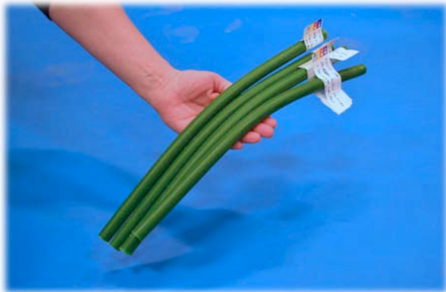
FIGURE 1. NanoSonic’s hydrogen delivery hoses demonstrating cryogenic flexibility
