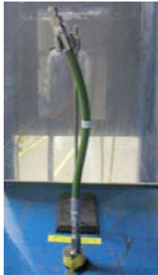
FIGURE 2. NanoSonic hose in hydrostatic burst strength test configuration
