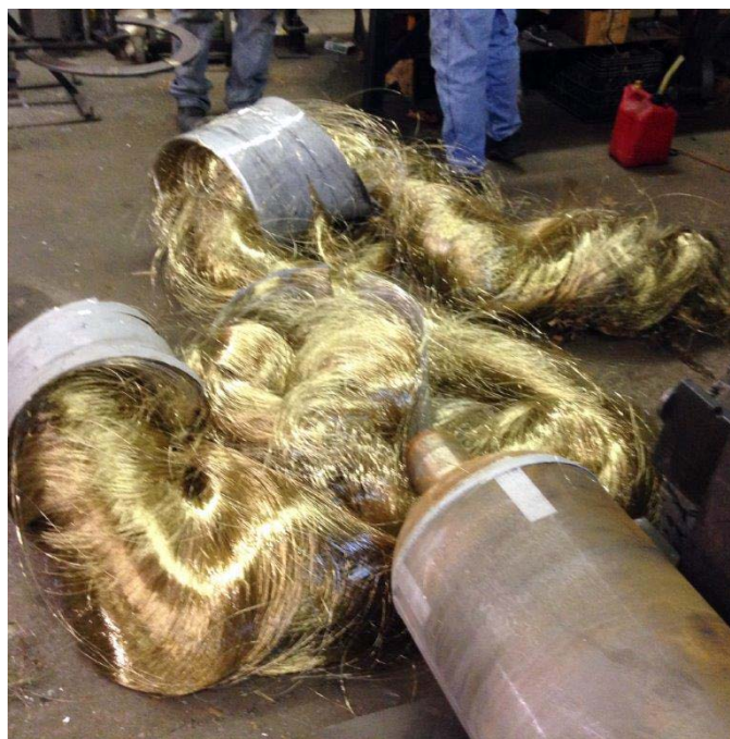
FIGURE 1. The condition of the liner after an attempted burst test during which the pressure was raised to 262.7 MPa (38,100 psi). Subsequently, the wires were cut to expose the surface of the cylinder. No visible sign of damage/cracking is seen anywhere on the liner walls.
