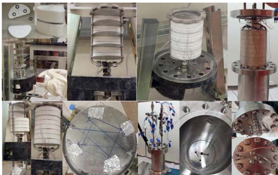
FIGURE 2. Various steps of assembly process and fully assembled flanged pressure vessel
