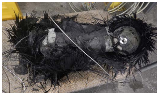
FIGURE 1. Image of burst tank made with vinyl ester resin
